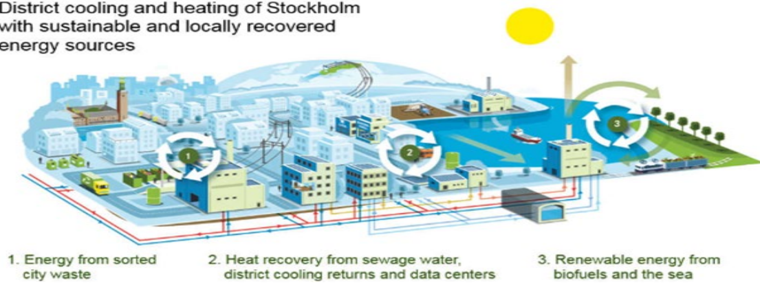
Figure 30 District cooling and heating of Stockholm with sustainable and locally recovered energy sources.[30]
