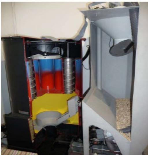
Figure 13 Pellet biomass boiler [14].
